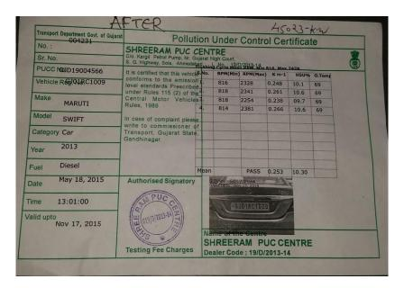
PUC test **after** installing ECO System – Drove 80Km at 6:50PM
